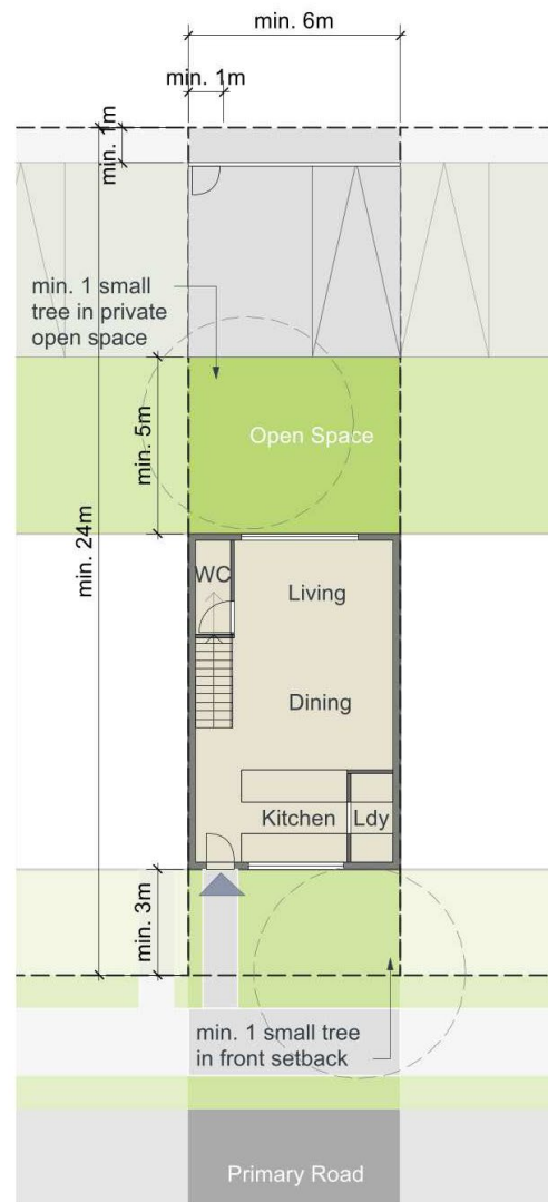
Figure 13 Rear-loaded townhouse plan
